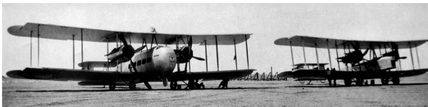
The capacious hull of the Vernon compared to the slim fuselage of its predecessor, the Vimy.
