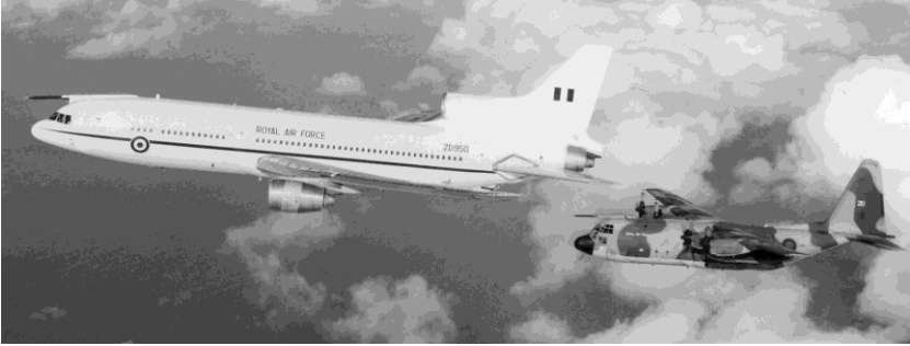
Hercules C1P undergoing receiver trials against a TriStar K1.
