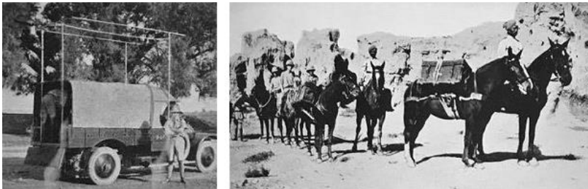
An improvised Crossley RAF R/T tender and an RAF cavalry R/T pack set.
