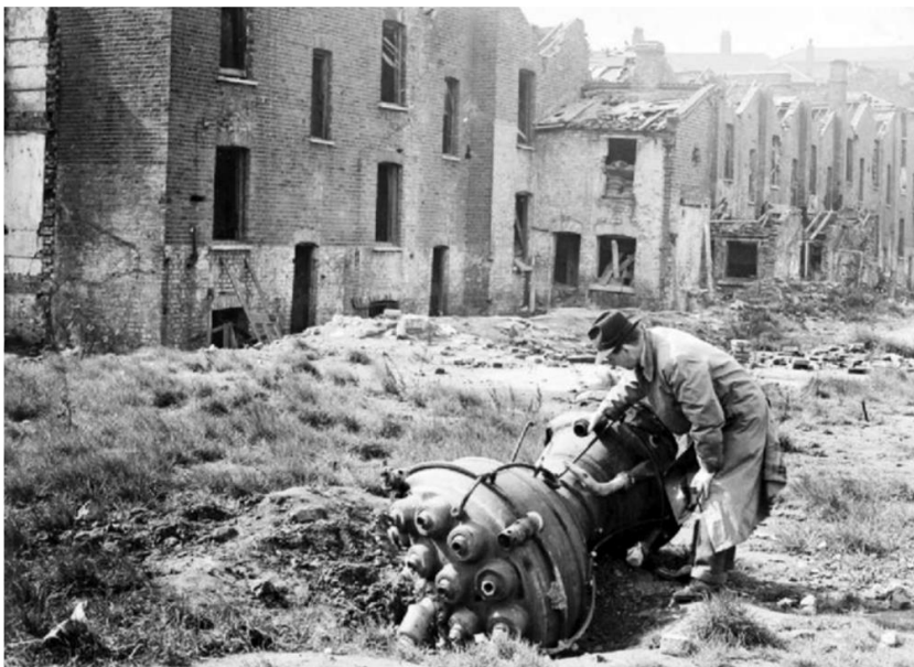
Chinatown (Limehouse, East London) V-2 combustion chamber and venturi which separated from a missile on impact. March 1945. http://www.wikiwand.com/en/Limehouse_Causeway
