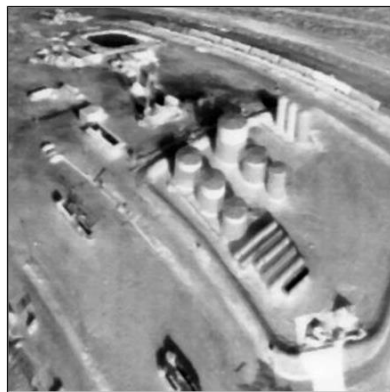
IRLS images of, left, the 'shadow' left by a P-3 Orion that had recently vacated its parking spot and, right, oil storage tanks revealing their content.
