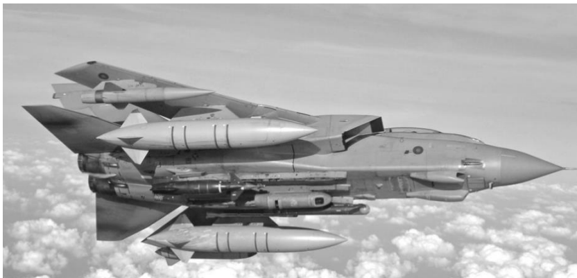
Tornado GR4, ZA589, carrying a DJRP on centreline under-fuselage pylon, an Enhanced Paveway II, on the right shoulder pylon and a TIALD pod on the left shoulder.
