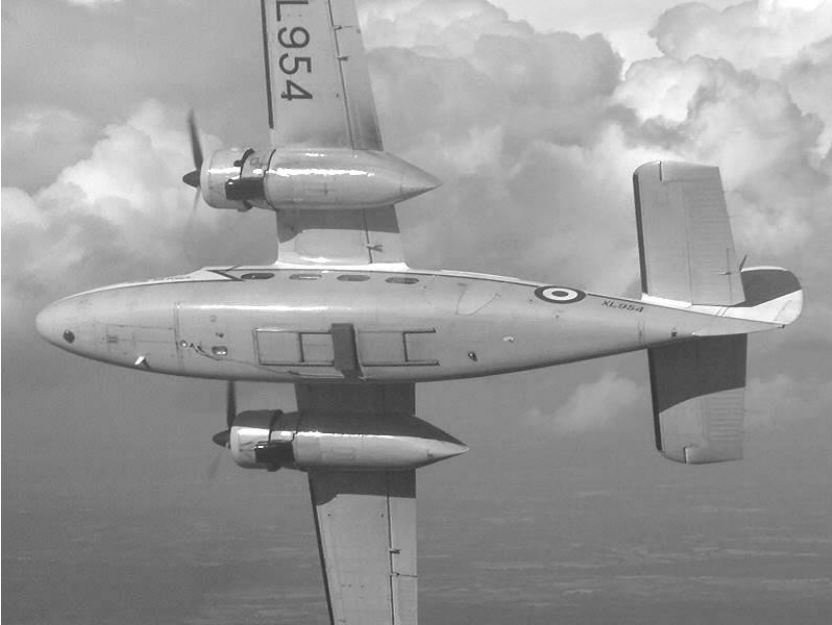
The camera hatches on the belly of No 60 Sqn's Pembrokes. Note that the second cabin windows (from the front) was glazed with non-refractive glass to aid photography using a hand-held camera.
