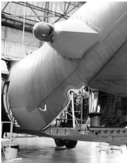
DIRCM installation on a C-130J.
