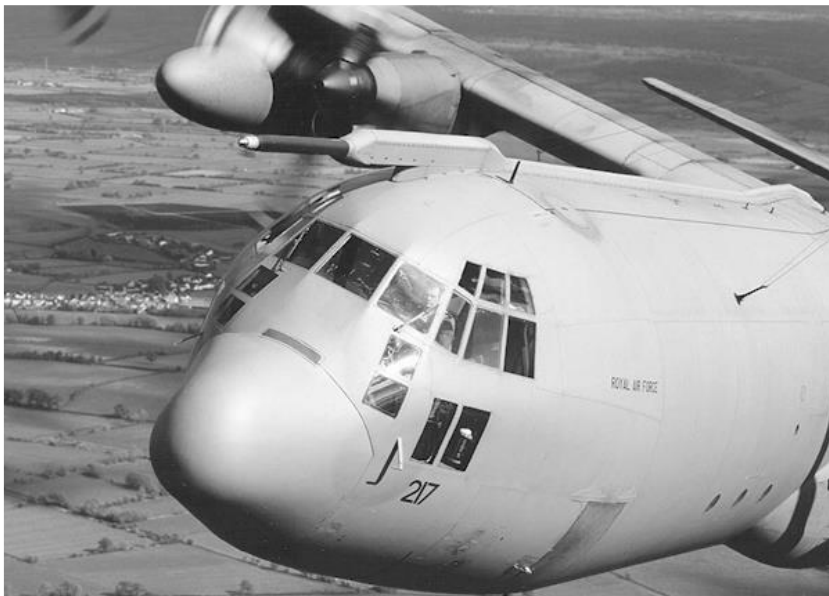
The C-130K-style probe and external pipe run.
