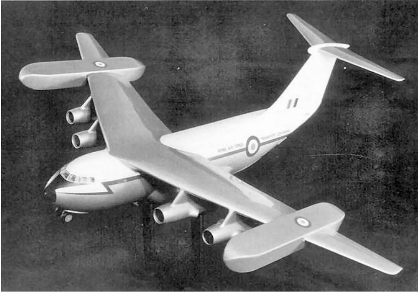
The AW681 in its twenty-two-engined VTOL fit . . . (BAe)
