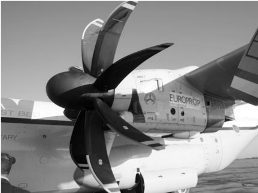
The A400M's Europrop TP400-D6 engine fitted to XV208.
