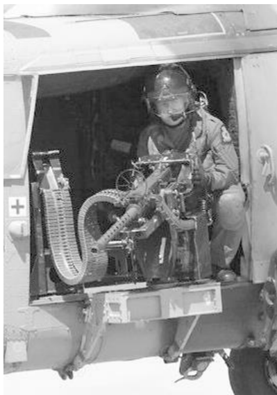
A 0.5 inch M3M machine gun mounted in a Lynx.
