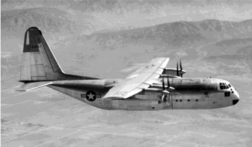
The YC-130 was distinguished by its snub-nose and 3-bladed props. (Lockheed)
