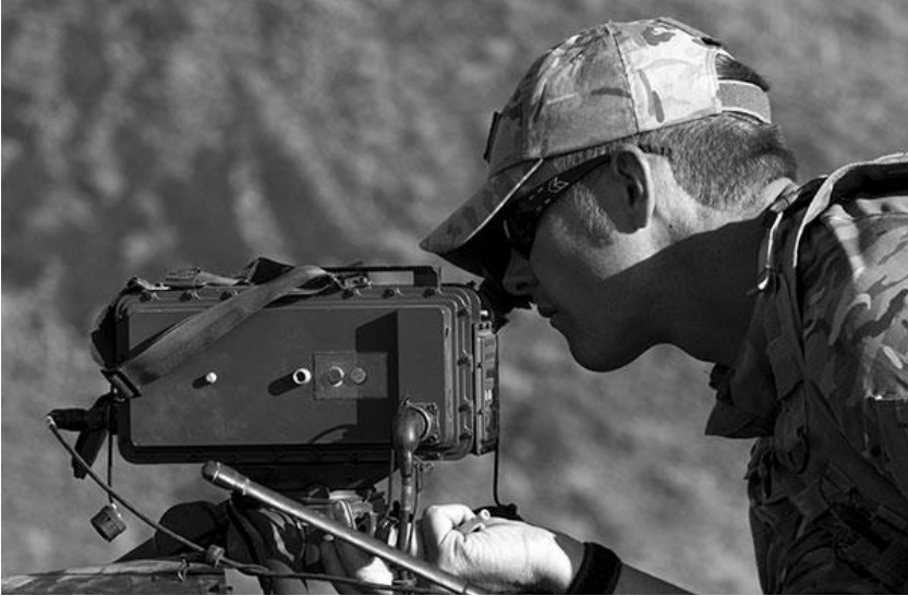
The use of laser designators, in this case by an Army JTAC, permits precision delivery of CAS.
