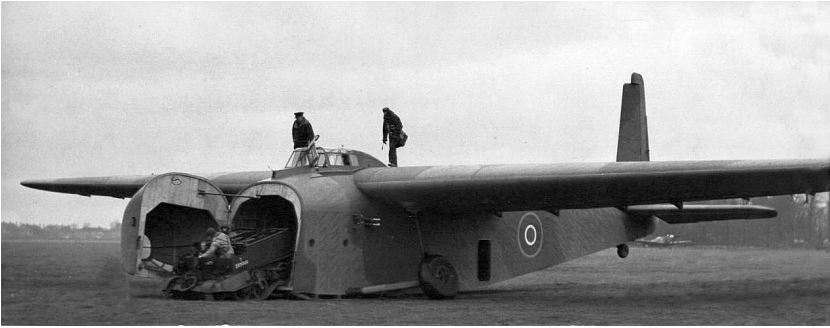
The capacious fuselage of the Hamilcar, with its swing-nose loading facility could accommodate quite substantial vehicles, in this case a Bren gun carrier, one of two.
