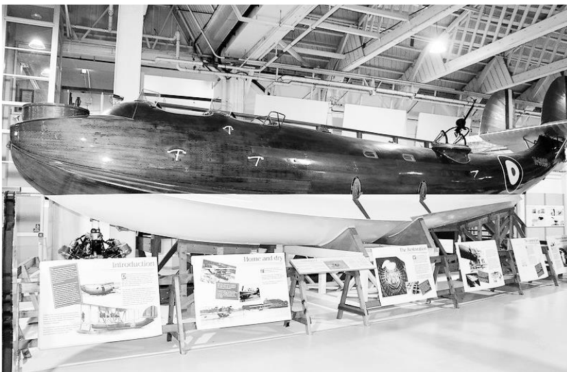
The RAF Museum's magnificently restored example of the wooden hull of an early Southampton, N9899.
