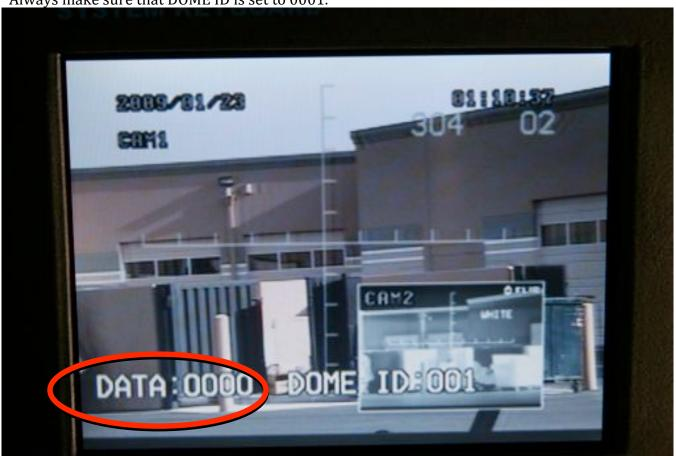
If DOME ID is not set to 001 the pan tilt will not respond. To correct this go into CCTV Video mode <FUNC> and <1> and then
