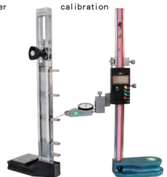
■ Step calibration of caliper
