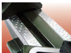
Precision grinding and scraping
