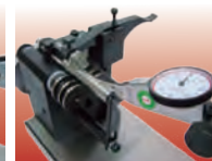
Example of measuring concentricity with indicator
