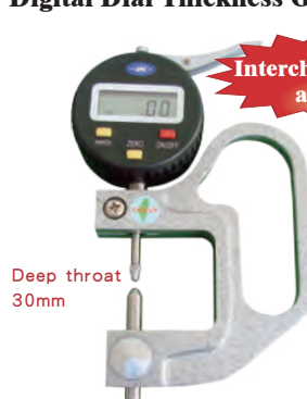
Resolution 0.01mm/0.0005" ET-9001GI 0-10mm NT$10230
