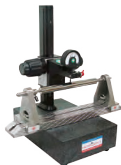
For measuring concentricity
