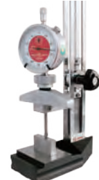
■ Depth gage calibration
