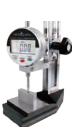
■ Digital indicator calibration
