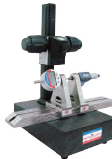
For calibrating varies type of dial indicators
