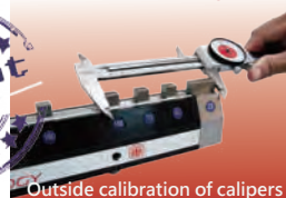
Outside calibration of calipers
