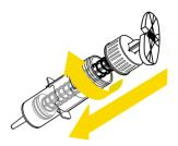
4. Insert the plunger into the body and screw it on the cap.
