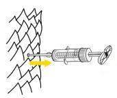
5. Once empty, unscrew the injector and cover the hole.
