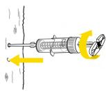
4. Screw the injector into the hole until it stops. Unlock by pulling the plunger and turning it 45°.
