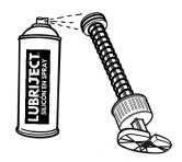
3. Directly apply a little amount of LUBRIJECT silicone spray on the O-Rings.
