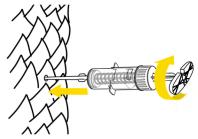
4. Insert the extender tip into the hole and unlock it by turning the plunger 45°.
