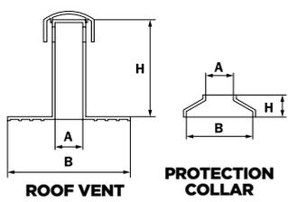
Manufactured of PVC, it is highly resistant against low temperatures (cold flexibility = -40°C) as well as perfectly compatible with any sort of PVC membrane. The flange is totally smooth for a perfect bonding to the waterproofing sheet. According to the length of 250 or 400mm, the spigot is provided with two or three couples of anti-infiltration rings.
