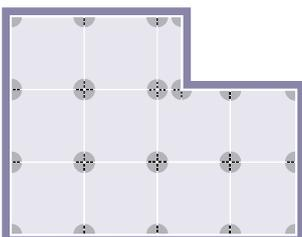
For pavers or tiles that are larger than 500x500mm, it is recommended that an extra paving support (with flat head) should be placed in the centre of the tile.
