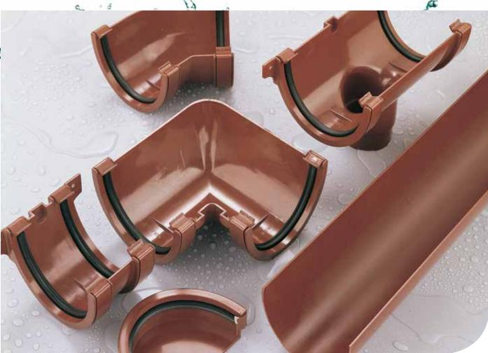
Deepstyle's high capacity nature provides a very efficient system for the drainage of large roof areas, whilst still providing a discrete unobtrusive rainwater system. In fact Deepstyle offers an increase of 50% in flow capacity when compared to the 112mm Roundstyle system.
