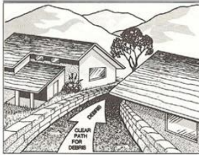
Figure 5: Directing Debris Flow between Buildings
