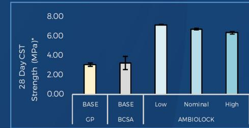
Figure 2. Performance comparison between compressive strength for stabilized sands. Note: all 32MPa concretes passed 32MPa hurdle (not shown here).
