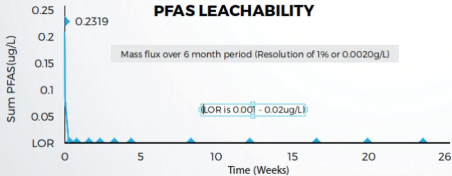
AMBIOPROTECT incorporated into a concrete substrate mix to achieve equal or greater material strength when compared to untreated concrete, restricting potential PFAS impact by up to **99%**.
