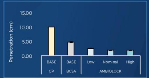
Figure 3. Performance comparison between permeabilities for stabilized sands. Note: BASE GP result exceeds measures (<10cm)
