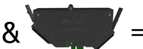
'Optical' SCD (Scatter Chamber Detector) 'Smoke' sensor
