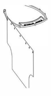
Align any extreme perforated hole on transparent face shield with the extreme Llatch of the forehead clip
