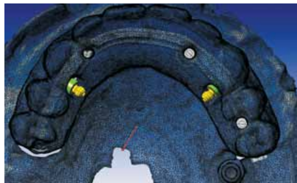
Fig. A A view of a CAM screenshot showing the virtually designed bar and threaded VKS 2.2 ball attachments.
