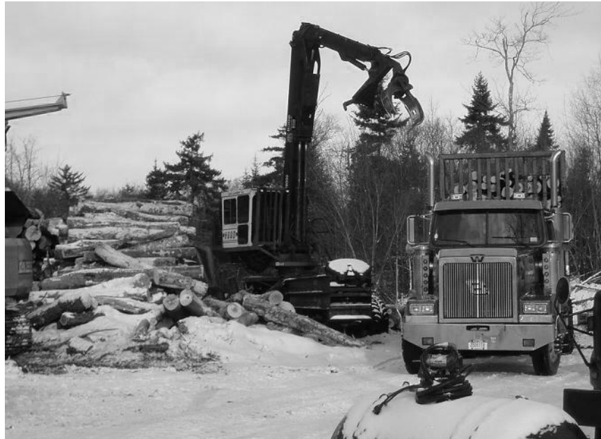
Hardwood pulpwood is cut into uniform lengths and then loaded on a tractor-trailer for delivery to the pulp & paper mill.
