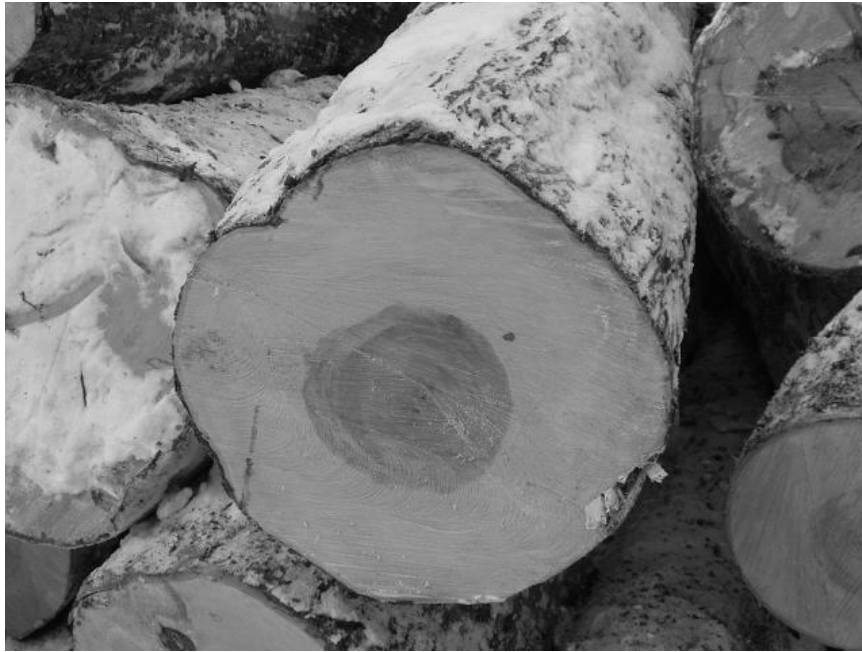
White wood and small hearts add to the value of hardwood sawlogs.
