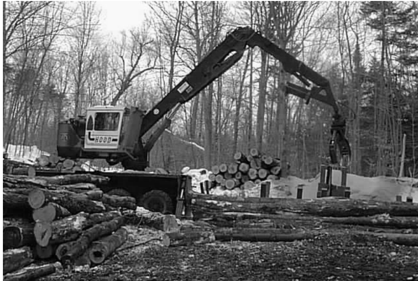
A log loader is often combined with a slasher for cutting tree-length stems into logs and pulpwood and then sorting and stacking them.
