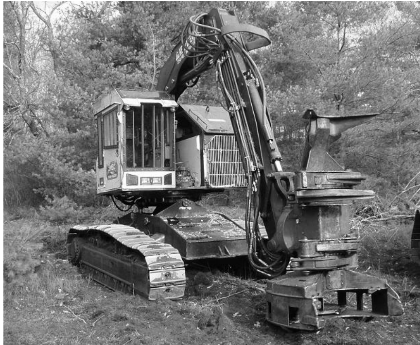
A feller-buncher is used to harvest trees and pile them for removal by a skidder or forwarder. This machine is equipped with an intermittent disc saw.
