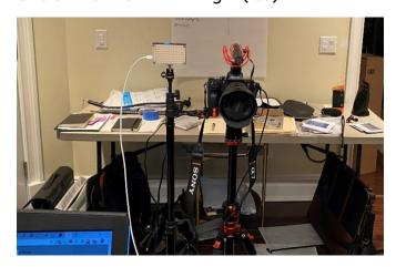
Apurture LED keylight (left of cam), Sony Z7RIII, RODE mic on top, (excuse mess under table)
