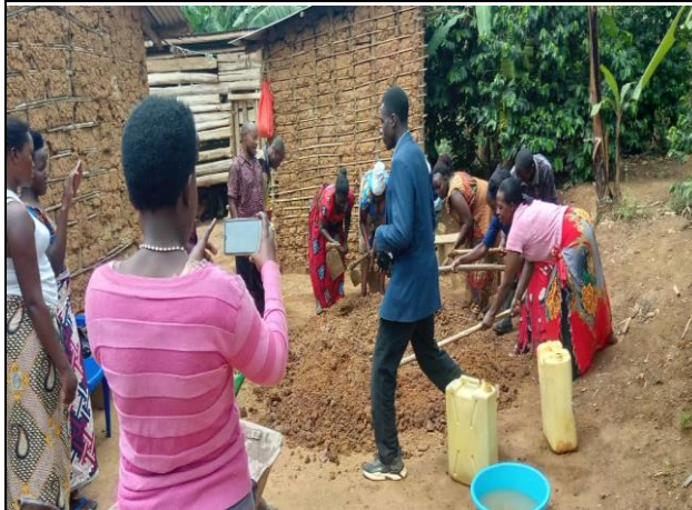
Women get involved to mix mud during training in making biomass cook stoves in Kitagwenda
