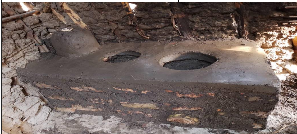
A completed biomass cook stove demo constructed at Butanda, Kabambiro Parish Kamwenge
