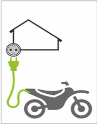
Mode 1: Ladestrom: 16A 1-phasig/ 3-phasig
