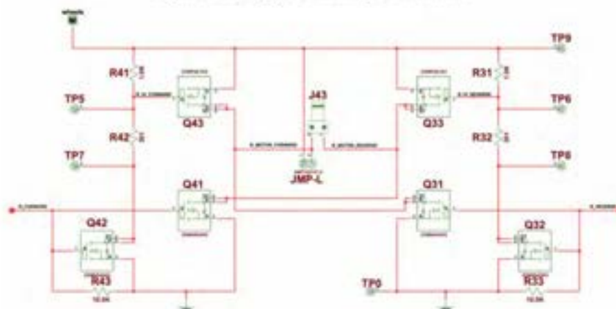
Figure 26: Left H-Bridge Schematic
