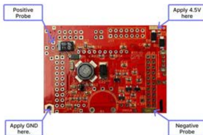
Figure 43: Annotated Power Board
