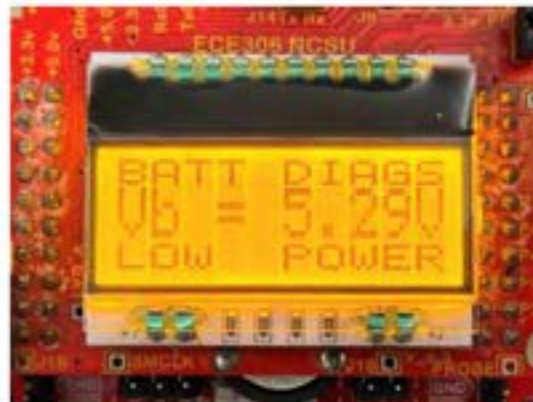
Figure 58: Battery Monitoring Display
