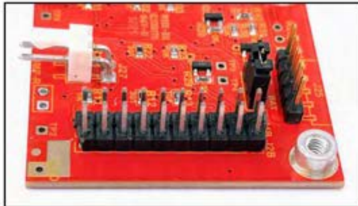
Figure 57: FET Board Replaced Header
