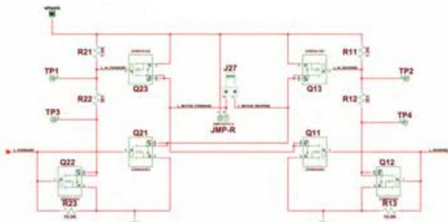
Figure 25: Right H-Bridge Schematic
