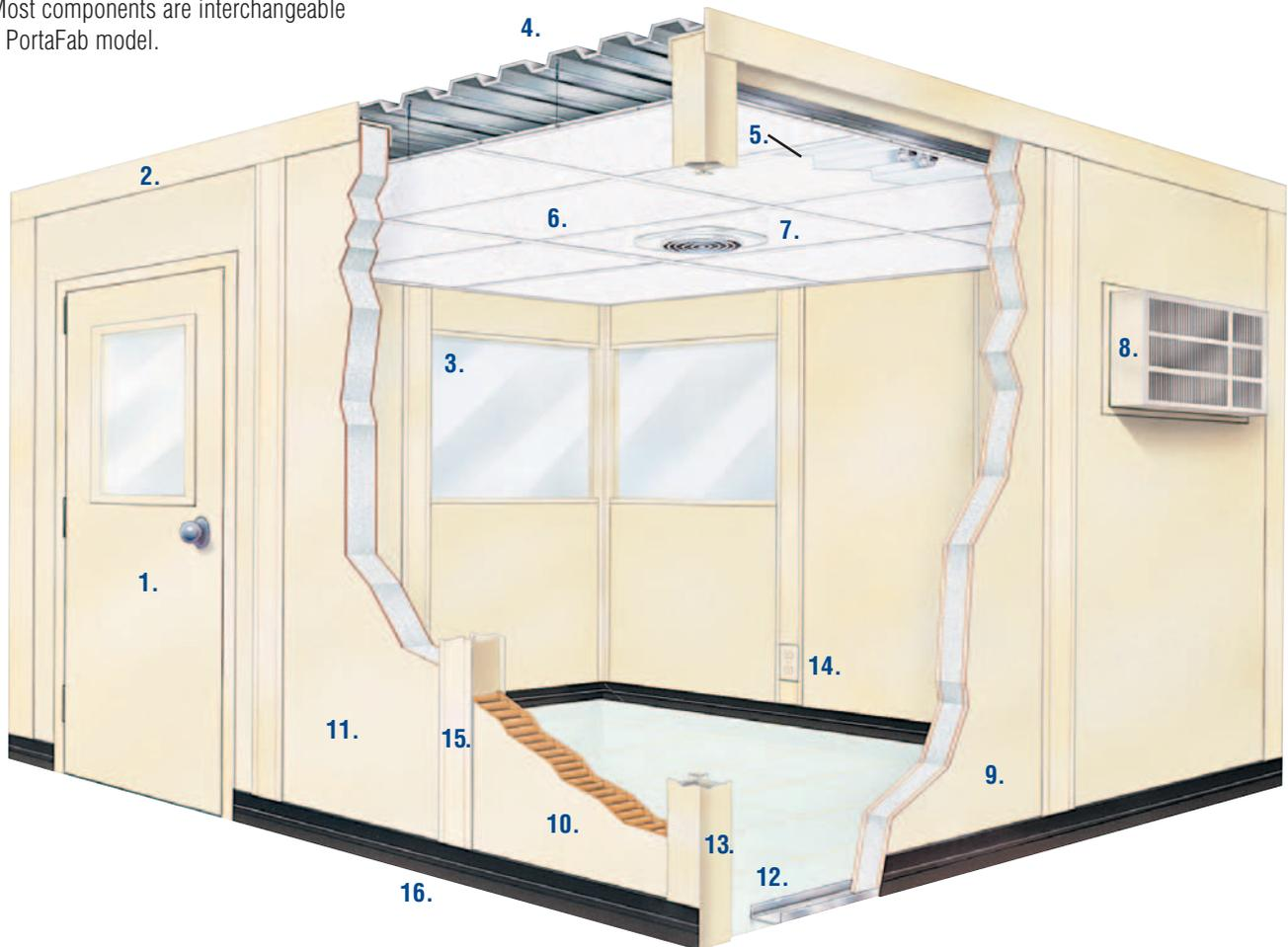
1. **3068 20 Ga. Steel Door** - 1 3/4" thick, comes pre-hung in frame; shown with optional glazing.
