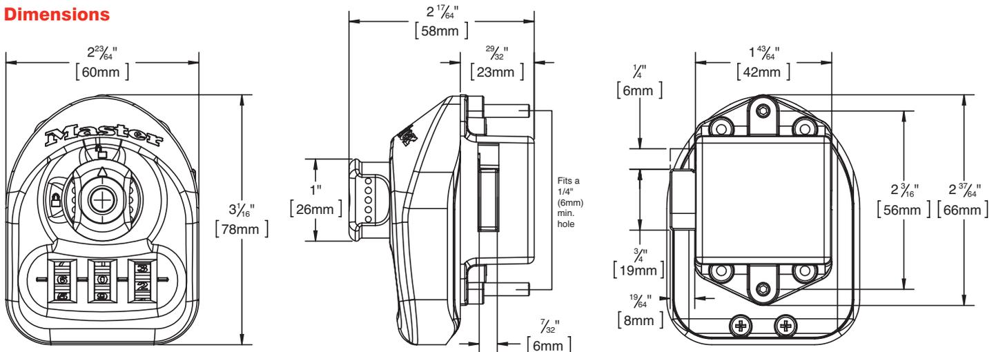
**Architectural Specifications:** Locks shall be built-in multi-user lock with models #3630, #3631 featuring vertically operating bolt and model #3670 featuring horizontally operating deadbolt. Locks shall have a disc cylinder for supervisory access. Locks shall have resettable combinations with no presets. Model #3630 for doors hinged on the left, model #3632 for doors hinged on the right and model #3670 for doors hinged on the right or left.
