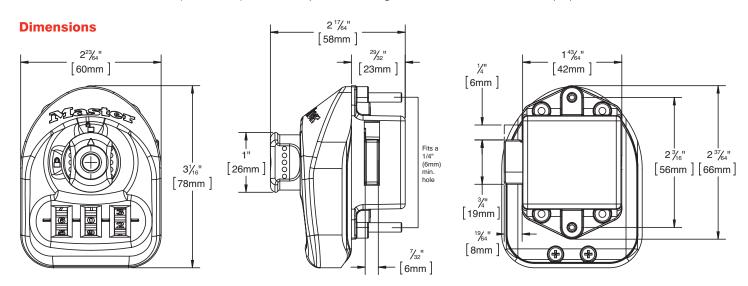
**Architectural Specifications:** Locks shall be built-in multi-user lock with models #3630, #3631 featuring vertically operating bolt and model #3670 featuring horizontally operating deadbolt. Locks shall have a disc cylinder for supervisory access. Locks shall have resettable combinations with no presets. Model #3630 for doors hinged on the left, model #3632 for doors hinged on the right or left.
