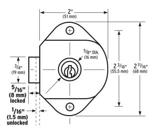
Architectural Specifications: Locks shall be key-operated with 5 pin tumbler cylinder with individual, group, or master keying [specifier must choose keying option]. Two(2) keys per lock and mounting hardware shall be included with each lock. Specify Master Lock #1710 for deadbolt operation or Master Lock #1714 for spring bolt operation. For optional master keying, specify Master Lock #1710MK or Master Lock #1714MK. For optional group keying, specify Master Lock #1710GK or Master Lock #1714GK.
