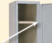
Magnum Student Lockers include a 3" wide 18 gauge full height door stiffener spot welded to the inner door face and MIG welded to the hinge side as well as to the top and bottom door flanges providing a rigid torque-free door. A 1-1/2" wide stiffener will be furnished for 9" wide Magnum doors.
