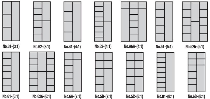
Widths for all-welded box locker openings 12", 15", 18"
