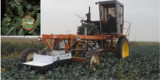
Figure 12. Selective broccoli harvesting with sensor technology on harvester
