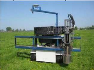
Figure 9. Image of an autonomous weeding robot
