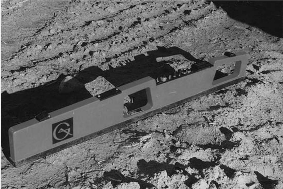
**Fig. B13.3.1** An example of a portable EM38 meter.
