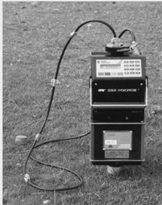
**Fig. B6.1.1** A neutron probe used for measuring soil water content *in situ*.
