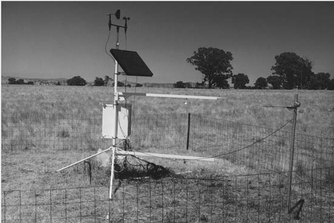
**Fig. B6.9.1** A field installation for measuring weather and other variables for  $E_e$  and the Bowen Ratio.
