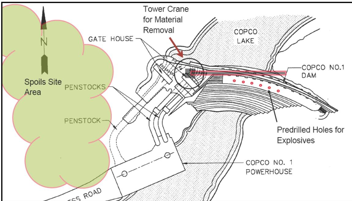
Figure 34 Copco 1 Dam Demolition Approach
