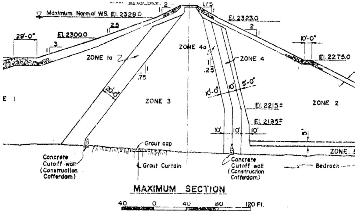
Figure 27 Section through Iron Gate Dam
