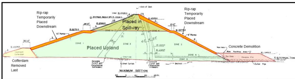
**Figure 25 Section Through Iron Gate Dam Showing Excavated Material Site Placement**
