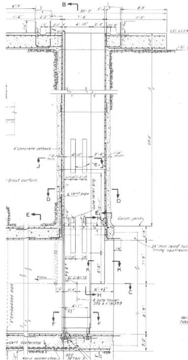
Figure 24 Section through Upstream Gate
