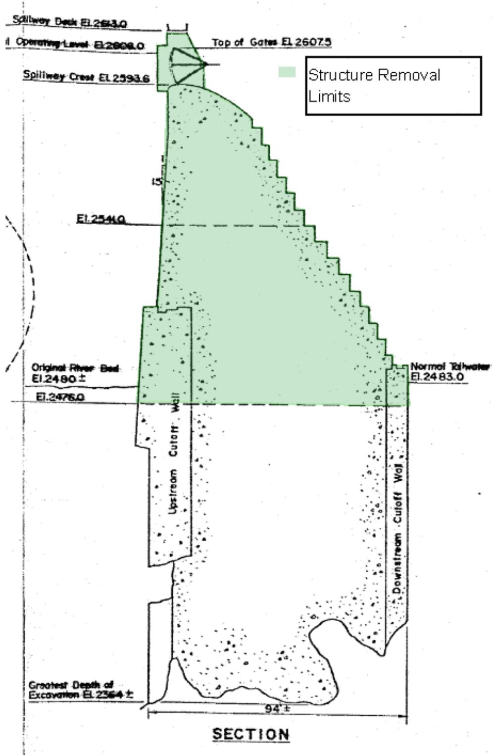
Figure 35 Original Drawing of Section through Copco 1 Dam
