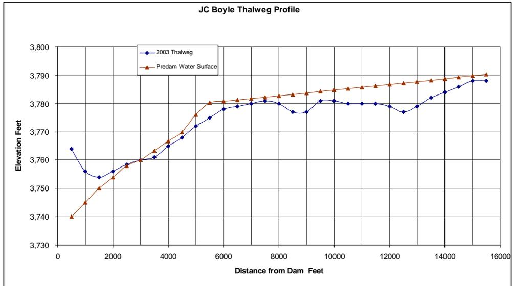
**Figure 44 Profile of Sediment in J. C. Boyle Reservoir**
