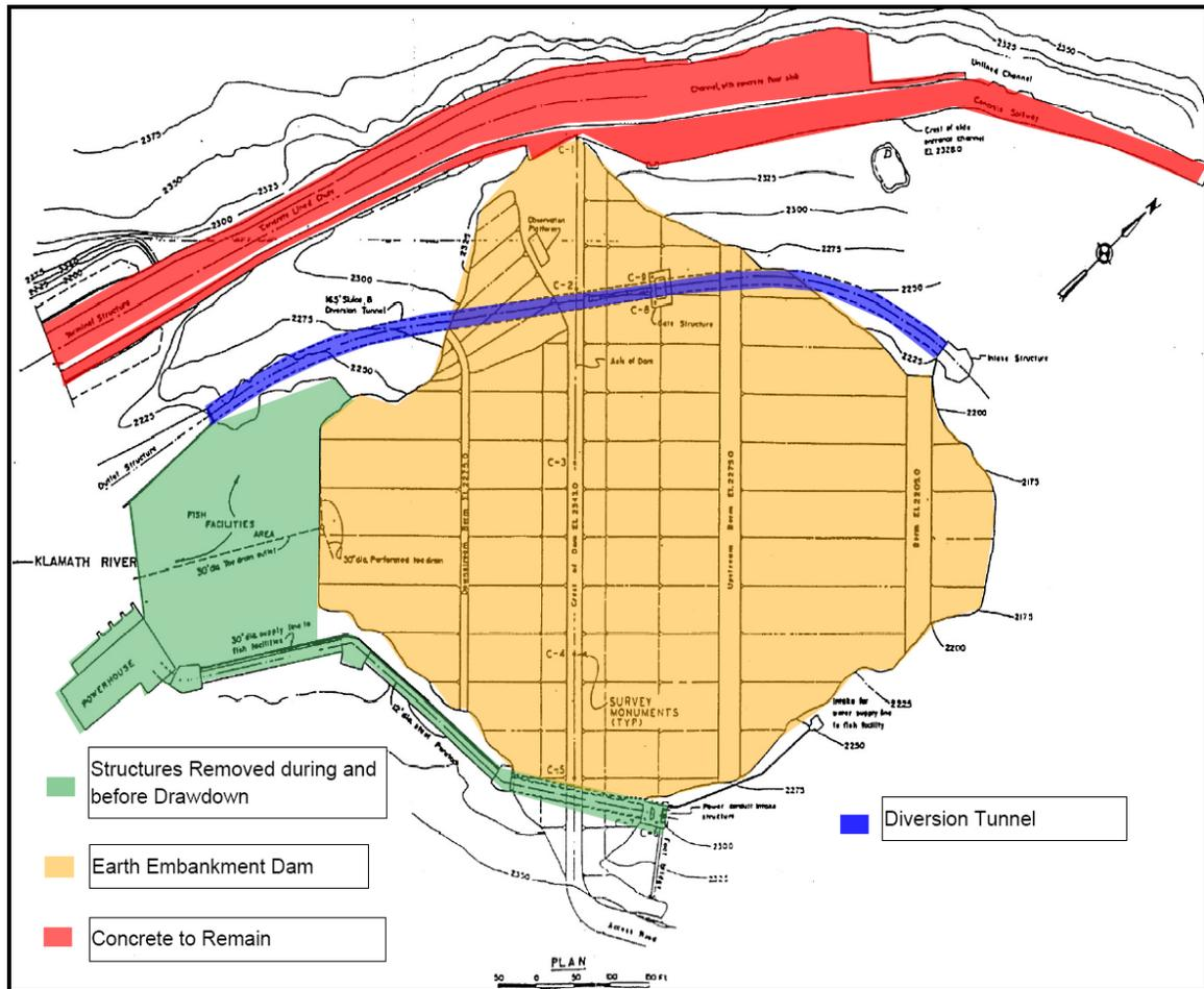
**Figure 26 Iron Gate Dam Structural Component Removed**
