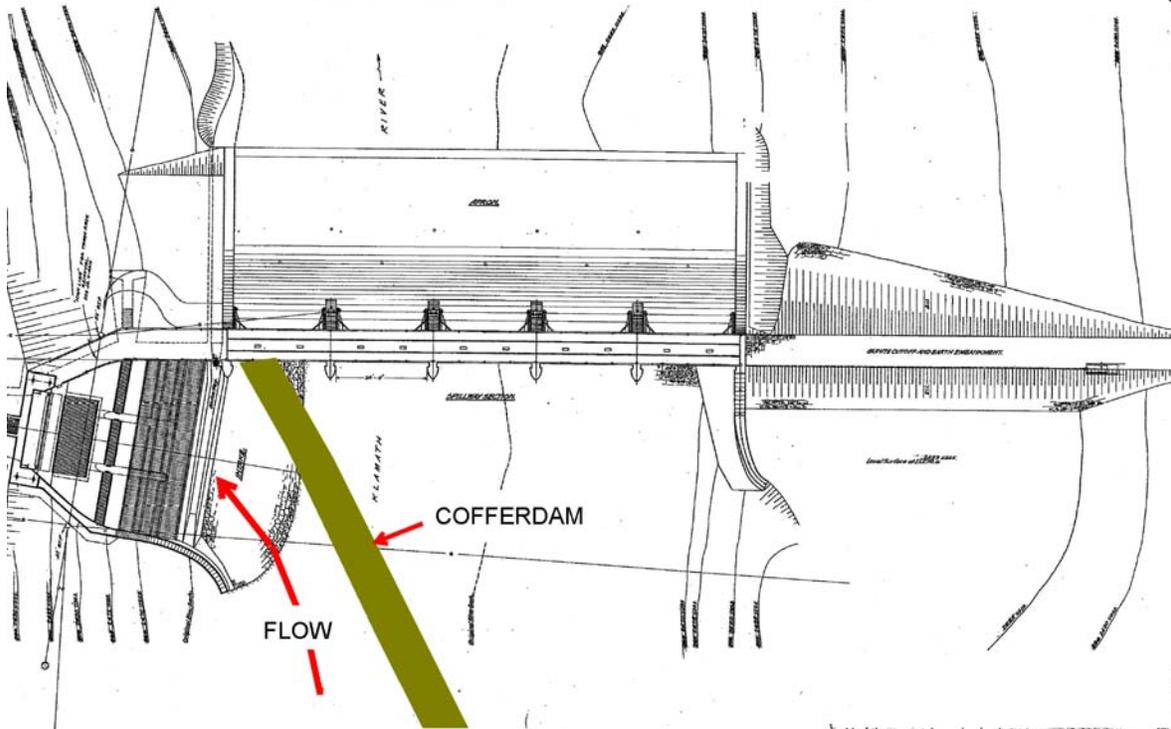
Figure 41 Cofferdam Diversion at Copco 2
