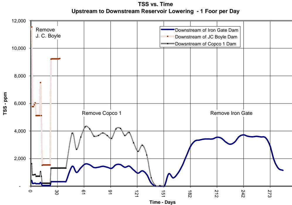
**Figure 15 TSS Resulting from Upstream to Downstream Removal**
