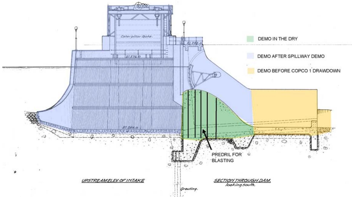
Figure 39 Copco 2 Spillway Removal Sequence
