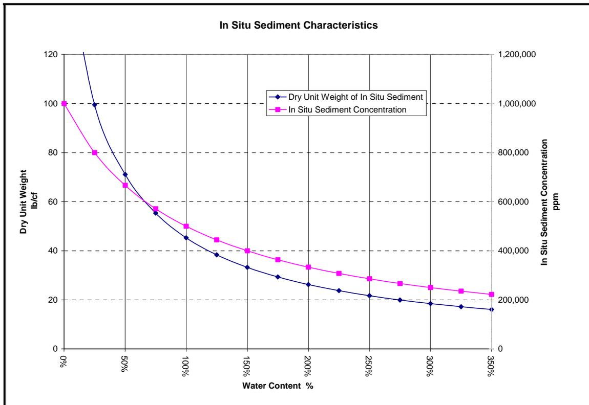
**Figure 10 Water Content versus Dry Density**
