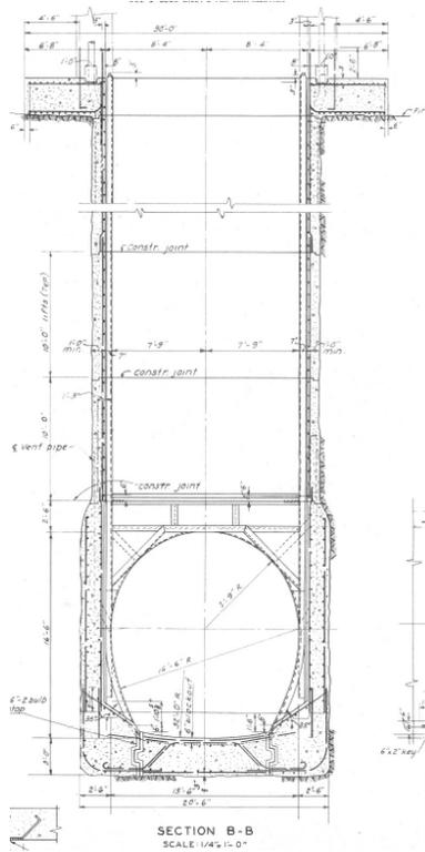
Figure 23 Section through Diversion Tunnel at Upstream Gate
