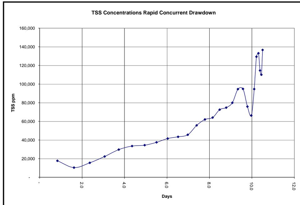
**Figure 17 TSS Downstream of Iron Gate for Concurrent Rapid Drawdown**
