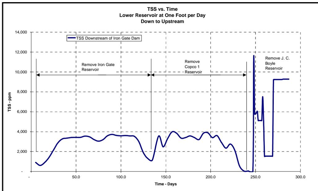
**Figure 16 Downstream to Upstream Removal**
