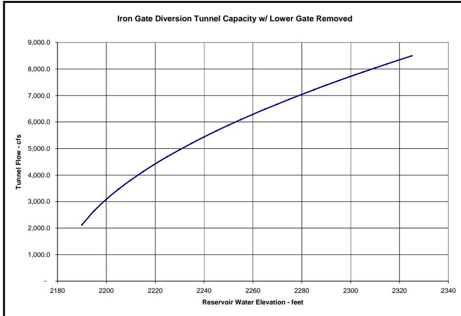
Figure 21 Iron Gate Tunnel Capacity Fully Open
