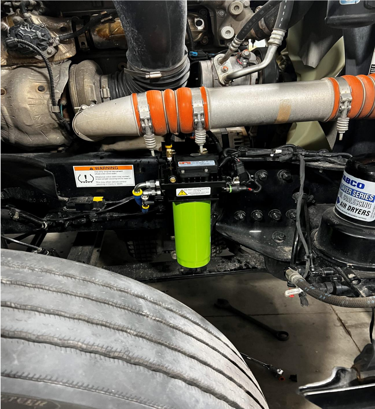
2022 Freightliner install DD15 with frame mounting bracket
