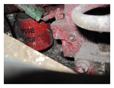
The picture below shows the supply port with the adapter and hose attached.
