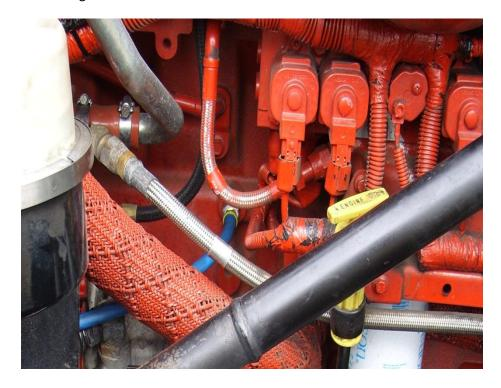
The picture below shows the return port. The drain plug is removed for this connection. There is a drain plug on both sides of the engine. The choice of which one to use should be determined by the mounting location. For example: If you mount on the right side of the truck, use the drain plug on the right side.
