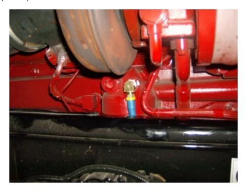
The supply port shown below is on the left side of the engine, just behind the air compressor. Use this port if you are mounting on the left side of the truck.
