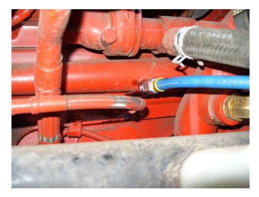
The port shown below is also on the right side of the engine. This port may be used, but is not preferred due to the proximity of the heated side of the turbo.
