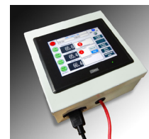
Remote Idec Control Panel
