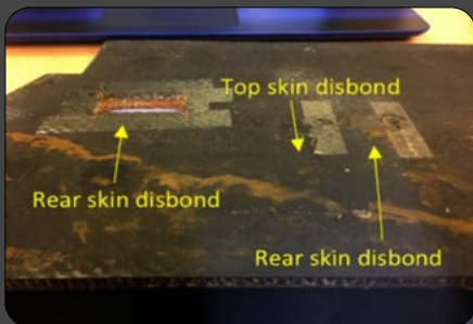
Figure 3: Thin CFRP honeycomb sample with rear surface disbonds.
