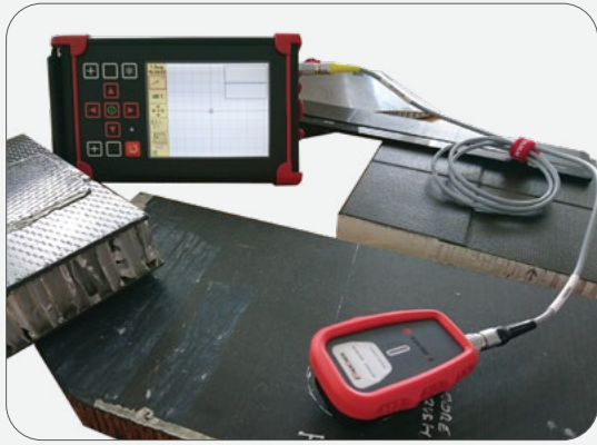
Rudder Probe: Pitch-Catch
