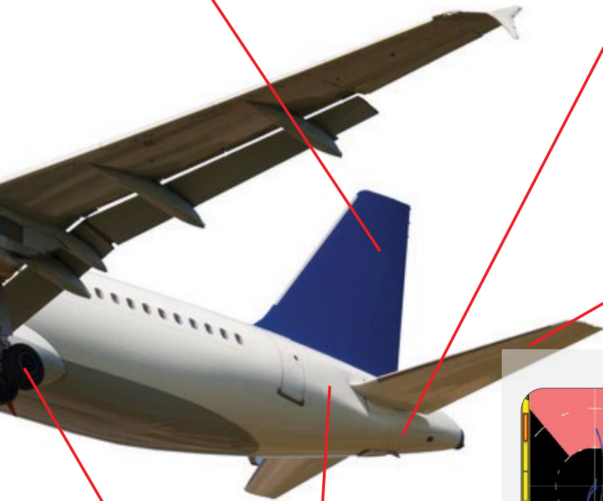
Area of Inspection: Horizontal Stabilisers Probe: High & Low Frequency, Pitch-Catch
