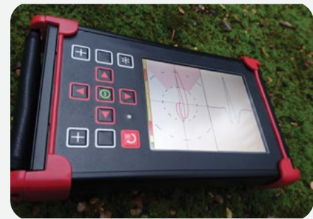
Area of Inspection: Horizontal Stabilisers Probe: High & Low Frequency, Pitch-Catch
