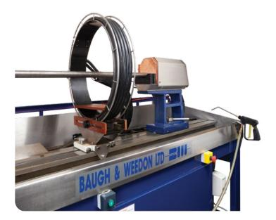
• **Remote Magnetising**. Components which are difficult to load because of their size or shape can be magnetised off the bench. Output sockets allow the bench power supply to be connected to prods, leeches or wrapped cables.
