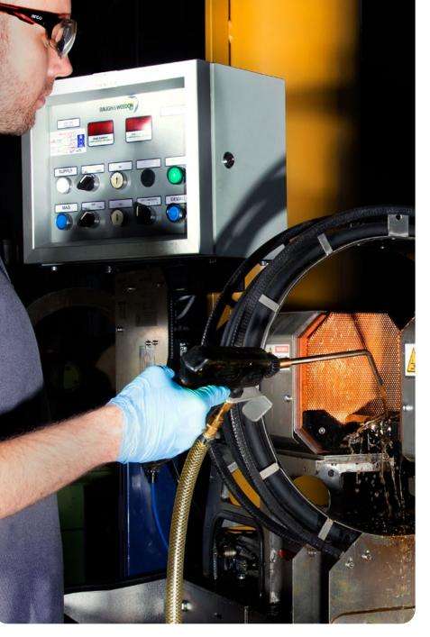
Baugh & Weedon Ltd is a trusted supplier of MPI equipment to the NDT industry. Their MAGAZON series of benches have a proven track record for reliability and durability, and are in daily use by most of the leading UK Aerospace companies. Designed and produced in Hereford, UK, the MAGAZON series offers testing for components of all sizes that require substantial magnetising currents.
