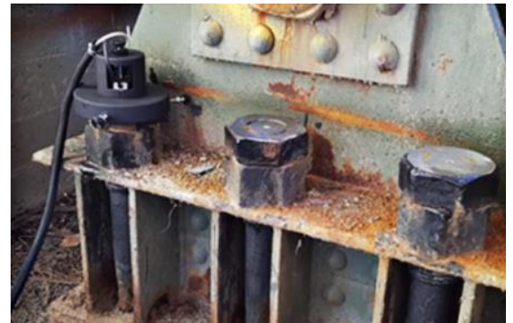
Switch clamp hubs to accommodate different bolt sizes or studs.
