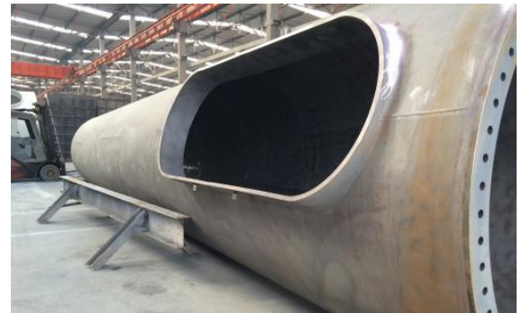
Complex weld configurations such as door frames or plate-bolt flange are made simpler with PAUT
