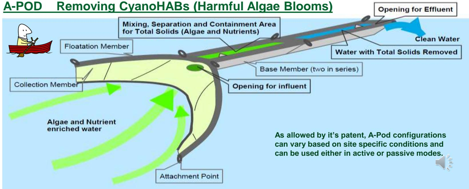
As allowed by its patent, A-Pod configurations can vary based on site specific conditions and can be used either in active or passive modes.
