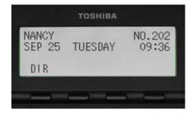
IP5000 4-line LCD display in Idle Mode
