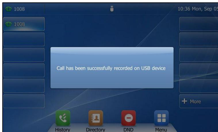
**Note** Unplugging the USB flash drive during a recording call will stop call recording, the recording will be saved on the USB flash drive automatically.
