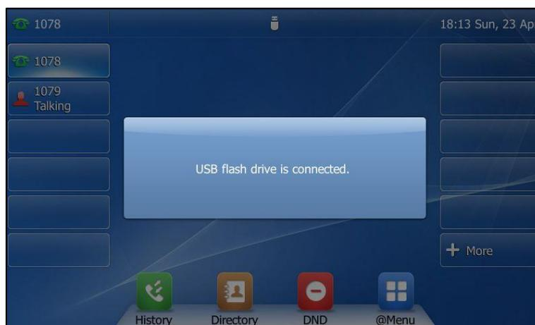
When there is an active call, and you insert a USB flash drive into the USB port on IP phone, the LCD screen will prompt "USB flash drive is connected. Remaining recording time: XX:XX:XX". For more information on the available recording time, refer to [Viewing the Storage Space](#) on page 201.
