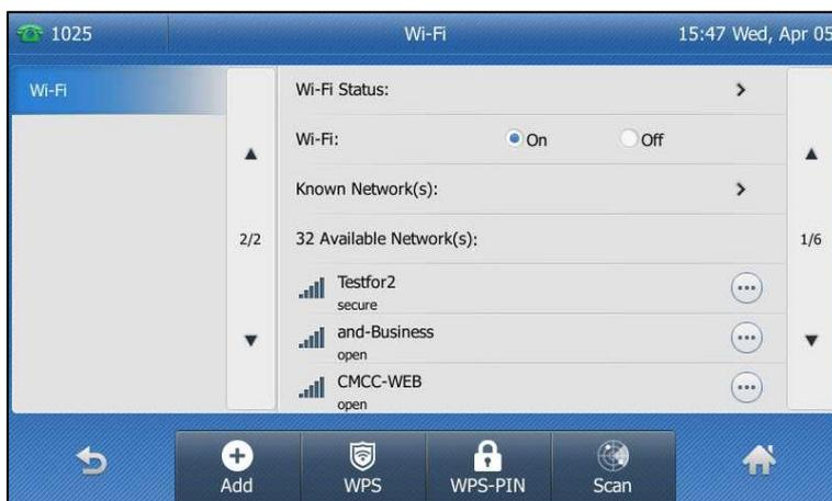
5. If the network is secure, enter its password in the **PIN** field.
