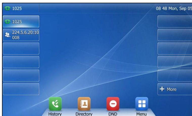
The following figure shows an example of label display when the label length feature is set to Default:
