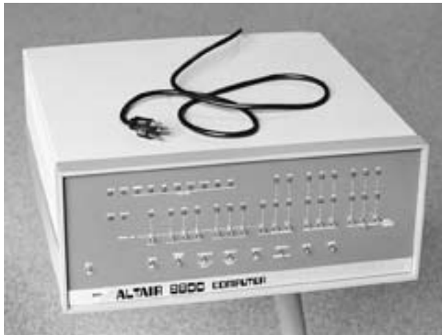
The MITS Altair (1975) was the first microcomputer available commercially. It was generally purchased in kit form. While the Altair did not have much processing capacity, it aroused great interest and inspired other computer builders such as Apple's Steve Wozniak and Steve Jobs. (CHRISTOPHER FITZGERALD / THE IMAGE WORKS)
