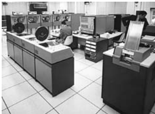
The IBM System/360 was the most successful mainframe in computer history. It was actually a “family” of upwardly compatible machines. (IBM CORPORATE ARCHIVES)
