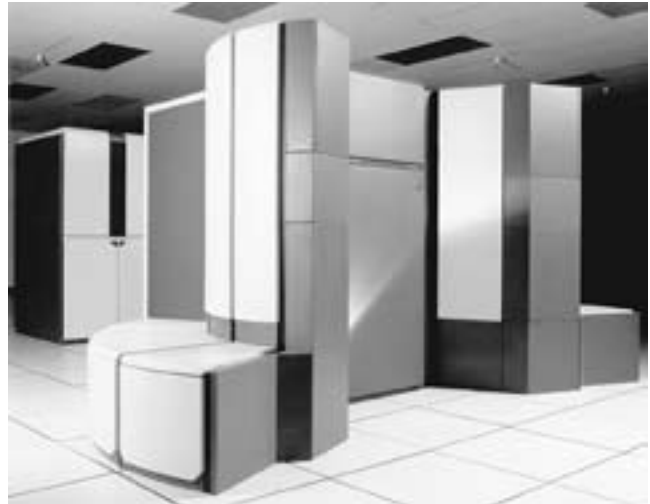
A Cray 190 A supercomputer. Seymour Cray's leading-edge machines defined supercomputing for many years. (NASA PHOTO)
