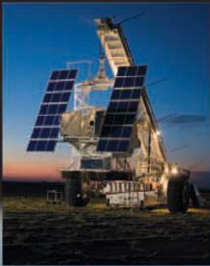
▲ THIS telescope was lifted by a balloon into the sky over the Arctic Circle. Since the Sun never sets there in the summer, the scientists could monitor the Sun all day.
