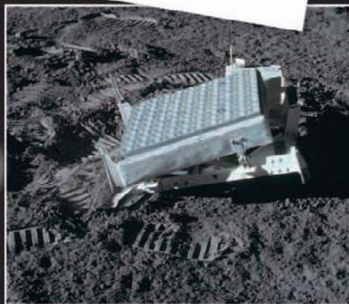
▲ SEVERAL reflectors have been placed on the Moon since 1969. The returning beams from the laser reflectors are too weak to be seen with the human eye and sensitive amplifiers are used to enhance the signal.
