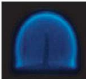
◀ SPACE FLAME In zero gravity, convection has no effect so flames burn with a rounded flame.
