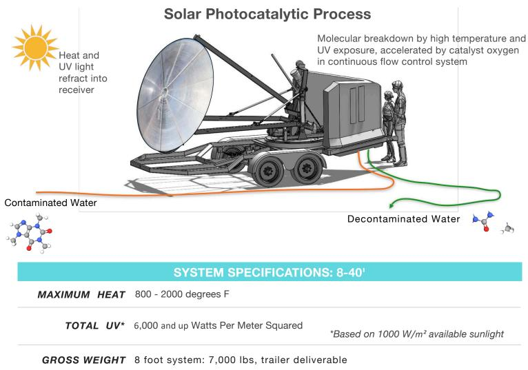
**THROUGHPUT** Up to 125 GPM. Variable, based on discharge requirements and affluent concentration.
