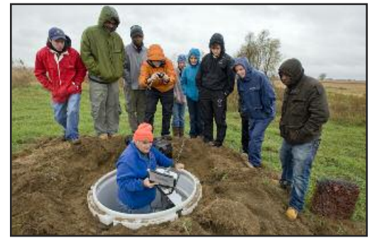
A group of students and researchers watch EarthScope Field Engineer Kenneth Oliver install a seismic station on October 19 near Kentland, Indiana. (Purdue University photo/Andrew Hancock)
