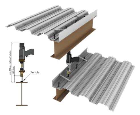
For all sections to receive welded studs, the top surface must be free of contaminants, paint and rust.
