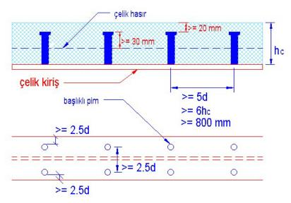
There are a number of rules and recommendations from approved design standards and industry best practice which specify spacings, dimensions and layout of studs in order to achieve the required stud resistance. Below is a selection of the most common examples.
