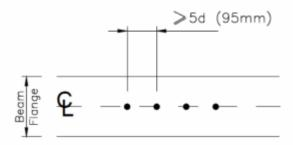
Single studs to be located on the center line of the beam except at butt joints where studs should be staggered in line with typical details, minimum spacings as indicated in Eurocode 4.
