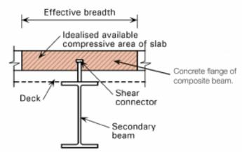
Steel designers design the steel frame to approved design standards (the latest being Eurocode 4). These design standards have formulae to calculate the amount of force that can be transferred by each shear stud. When designing the composite beams, the steel designer will calculate how many studs are needed for the beam design based on these values.
