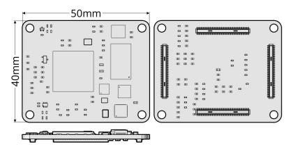
The XLM42 and XLM43 series features Efinix® Titanium® FPGAs packaged in a 4cm x 5cm module. Additionally, the modules contain on-board:
